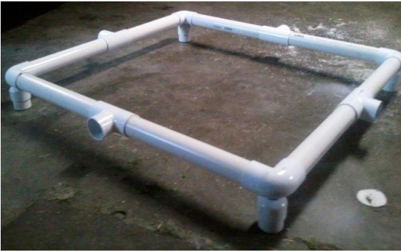
Figure 7; Pig rails made from PVC pipe
